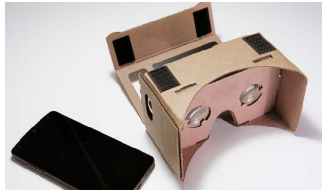
Figure 4: ‘Google Cardboard’ VR headset with opened phone compartment. The mobile phone on the left is inserted into the compartment with the display facing the lenses.
